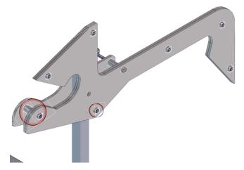
**Step 14**: Secure the assemblies together with a 3/8-16 Nylock Nut (am-1054.) Do not over tighten. The Hook Assembly should still easily pivot.
